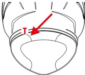
2 Slide the pipe between the check pad and the internal part of the helmet, following the trim at the bottom.
