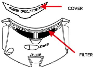
3 Refit the cover by plugging and pressing the hooking teeth in the appropriate houses and make sure that the cover is completely hooked to the chin.
